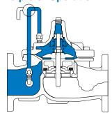
**Tight Closing Operation** When pressure from the valve inlet (or an equivalent independent operating pressure) is applied to the diaphragm chamber, the valve closes drip-tight.
