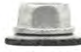
Correct Installation Tight against surface. Seal flows inward to seal minor fastener diameter and surface voids
