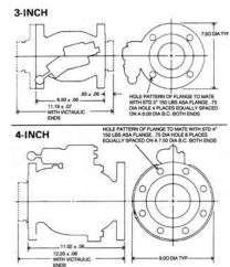
Meggitt manufactures 3-inch and 4-inch bottom loading shutoff valves for use with either the jet level sensor or float pilot valves. Refer to pages 602 and 613 for complete details on pilot controls. Both sized valves are available with ASA 150 pound flanges or ends to mate Victaulic couplings and are made of aluminum. Both valves are also available in Ductliron.
