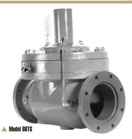
The Model 66TS Tank Safety Valve is designed to automatically isolate a fuel storage tank from its loading terminal or product transfer point. Hydraulically linked to the delivery pump, the valve is open only when the pump runs and is effectively producing pressure. The valve will automatically close when the pump is off, fails to produce pressure, or in the event of a line rupture.
